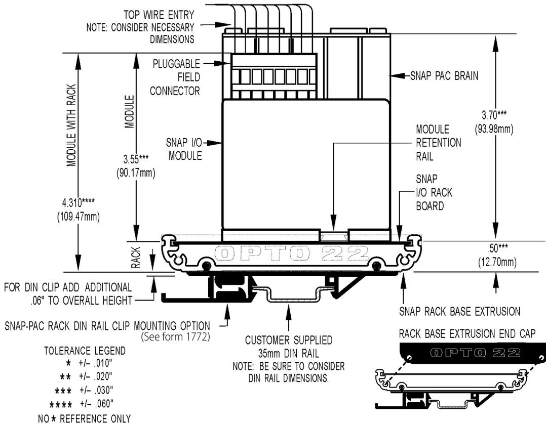
For more information on DIN-rail mounting kits, see form 1772, the *SNAP TEX Mounting/Wiring Tools and Spare Parts Data Sheet*.
