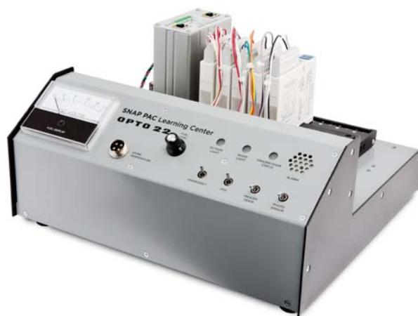
The course uses a learning scenario of a fictional convenience store, with digital input and output devices (lights and door contacts), and analog inputs and outputs (fuel sensors and displays).
